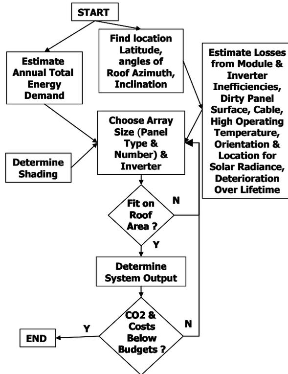
Figure 4 - Zero Carbon PV System Design Method
