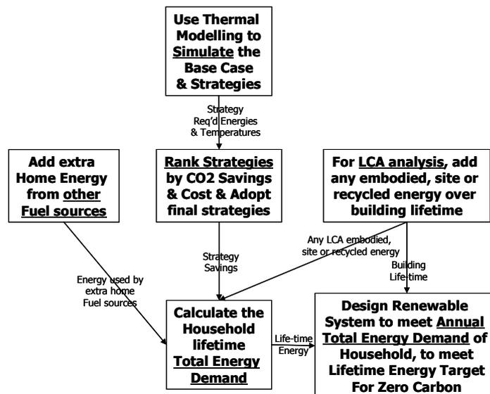
Figure 3 – A Method for Practical Zero Carbon Refurbishments
